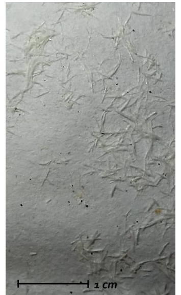
Figure 2: Rejected fraction of the repulped material: large fibres, grey, shiny and coloured specks
